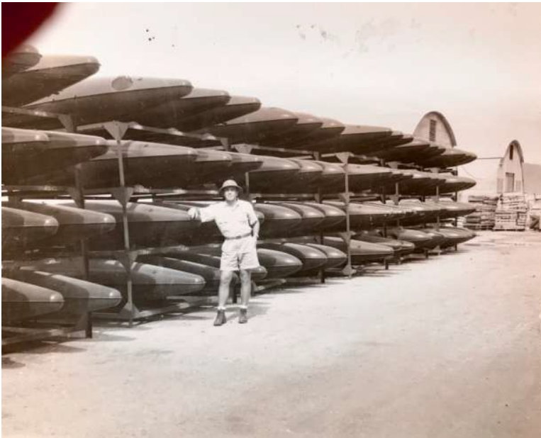
George Jedenoff inspecting the finished product – 175 gallon droppable fuel tanks
